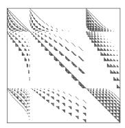
Though the polynomial p has many monomials, only 11% of the coefficients of the matrix S are not zero. There are 21 singular points on this curve (which are all real), and by this method we are able to select the point whose first coordinate is the nearest to 4. Notice that the matrix of multiplication by this linear form in  $\mathcal A$  can be computed by solving 21 systems associated to the matrix S.
