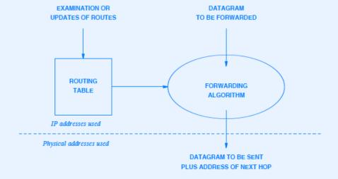
Routing table uses IP addresses, not physical addresses
