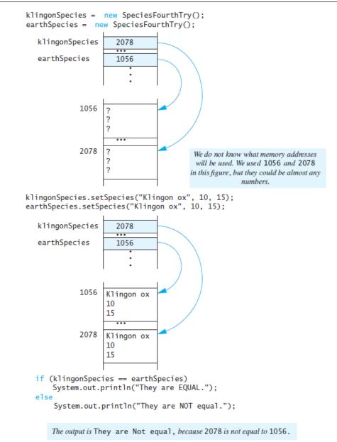
FIGURE 5.6 The Dangers of Using == with Objects
