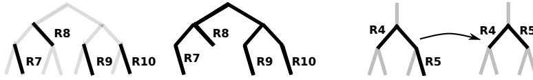
Fig. 2. Left: Given a configuration of leaf labels on an airway centerline tree, extract the subtree spanning the leaf labels and prune off the rest, giving the subtree spanning the labels , a geometric leaf-labeled tree which can be compared to the training data. Right: After assigning a set of labels, each label is moved to the branch in the segmented airway tree closest to the root which is not part of the subtree spanning the other labels.
